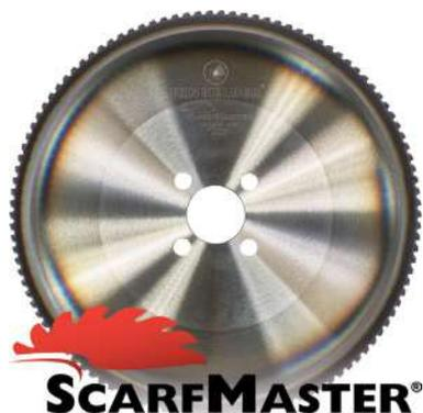
The PVD coated carbide tipped ScarfMaster has specifically been designed for flying cut-off applications dealing with heavy inside scarf. It features a very specific tooth geometry, combined with highly shock resistant carbide tips.
